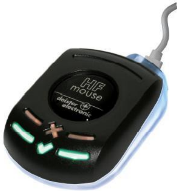
Slika 4: Čitalnik RDL5 – HF RFID – Mouse (Vir: http://www.deisterrfidportal.de/_docu_pdf/rf_rd15_eo.pdf )
