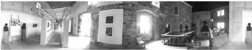
Figure 6. 360° panoramic image generated with only one horizontal scan out of 200 images using a wide angle lens.
