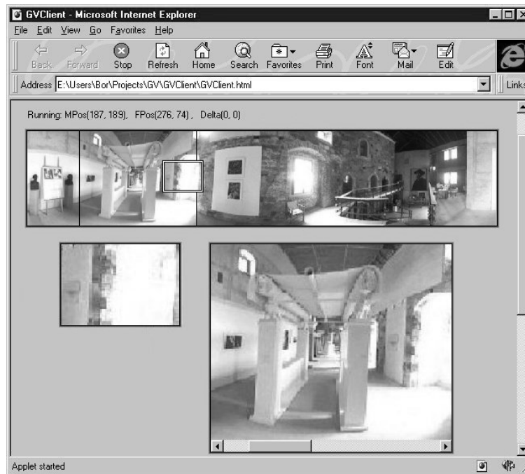
Figure 7. GlobalView interface of IVS. The rectangle in the panoramic image indicates the attention window which in turn indicates the current direction of the camera. By moving the rectangle the user controls the direction of the camera. On the bottom of the web page the live video image in actual resolution (left) and a zoomed panoramic view (right) are shown.
