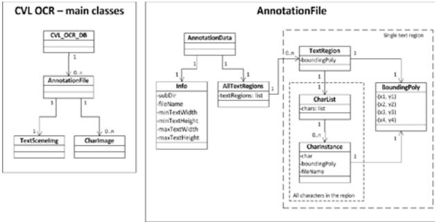
Fig. 4. The CVL OCR DB conceptual model.
