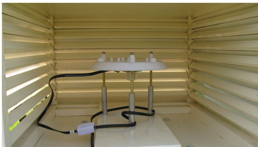
Slika 2.2: Senzor temperature in vlage (termometer in higrometer).
