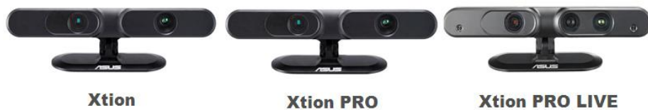
Slika 4: Senzorji gibanja Xtion, Xtion PRO in Ktion PRO LIVE.
