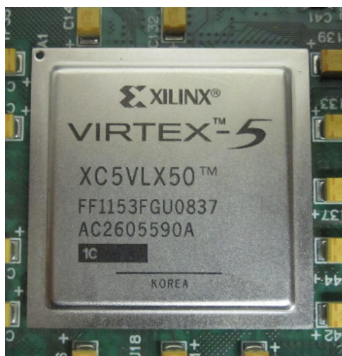
Slika 3.2: Xilinx Virtex 5 XC5VLX50
