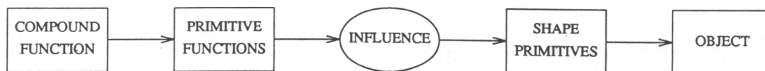
Figure 1 Synthesis procedure for design of objects. Function or purpose that define the basic category dictate the part configuration and the shape of individual parts.
