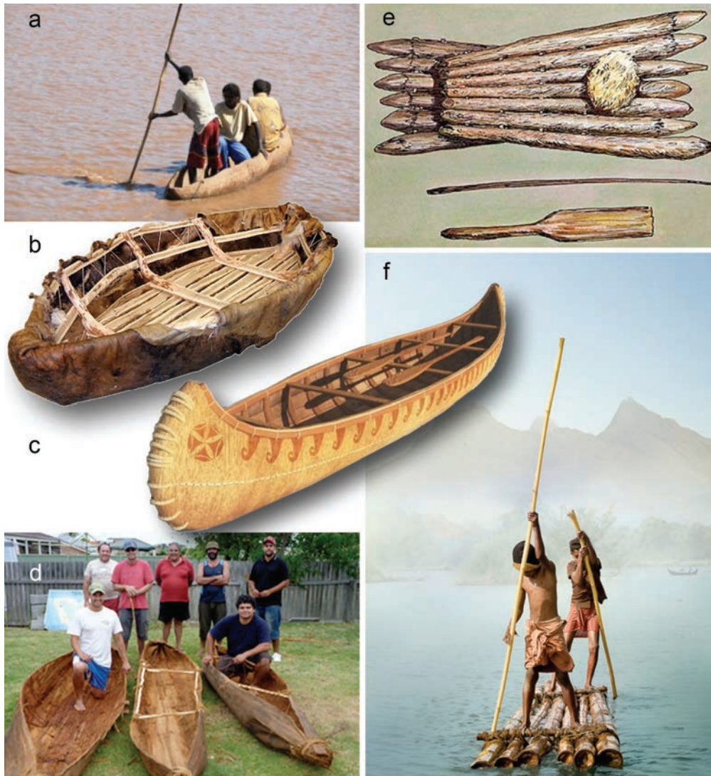
Figure 3. a. Logboat on “Omo-Bottego” River, Ethiopia (Photo: Peter and Hinda Schnurman) [15]; b. Angyaqatak Skin Boat made 2007 by Joe Spein and Alexie of Kwethluk. [16]; c. Native Americans bark/skin boat originally called dugout [17]; d. New South Wales south coast, Australia. Workshop participants with their tied-bark canoes (Photo: David Payne/ANMM) [18]; e. Double triangular raft from Western Australia (Illustration: Xiangyi Mo) [19]; f. Bamboo raft from Kerala, India (Photo: Enjo Mathew) [20]
