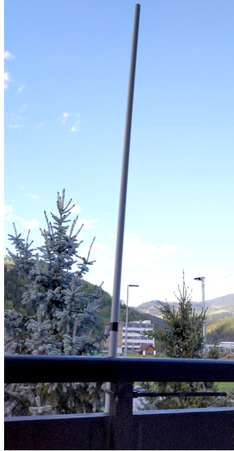
Figure 4.2: Hardware capturing setup: custom made colinear dipole 1090Mhz antenna
