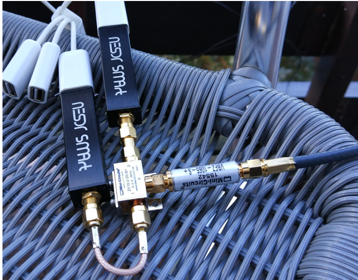
Figure 4.1: Hardware capturing setup: 1090Mhz filter, signal splitter and two SDR dongles
