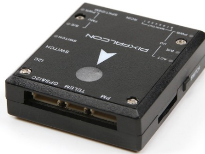
Figure 3.3: An image of the PixFalcon FMU. Image source: holybro.com
