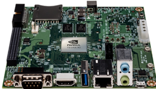
Figure 3.5: NVIDIA Jetson TK1 embedded developer kit. Image source: nvidia.com
