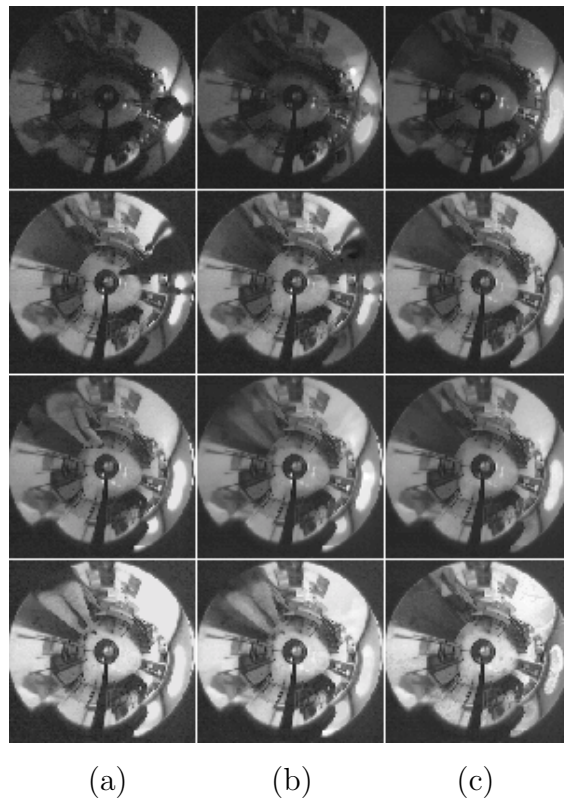
Figure 5.6: (a) Four panoramic images from sequence. Their reconstructions based on (b) standard PCA, and (c) robust PCA.
