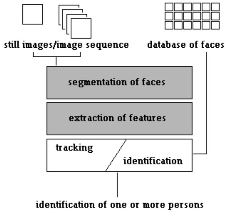
Figure 1: Machine face recognition algorithm
