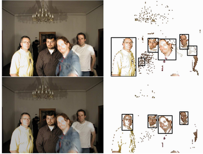
Figure 5: Retinex performance: In the upper part of the figure we see two false detections, while on the lower part this problem was overcome by the Retinex algorithm. The image was taken from the flashlight subset.
