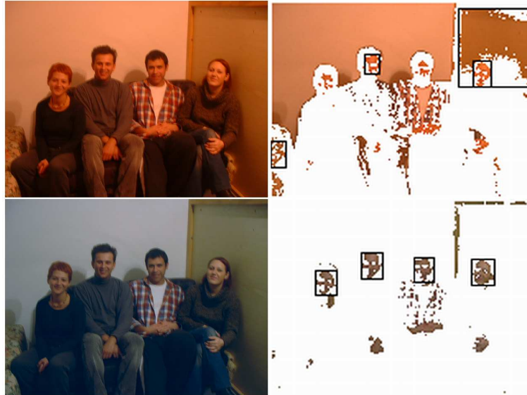
Figure 6: Correlation performance on image from the yellow subset: detection results on image without preprocessing (top) and after illumination reconstruction (bottom).
