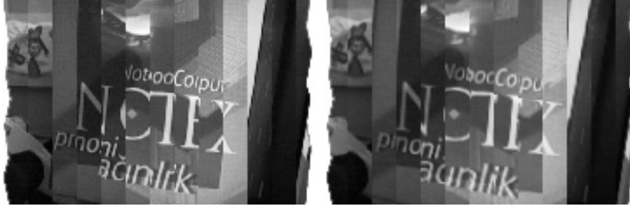
Figure 3.12: Parts of panoramic images from distorted (left) and undistorted (right) sequence of images. We can see that the problem with missing scene points in the panoramic images (Sec. 3.2.1) remains. Compare the images with the image presented in the bottom of Tab. 3.4.
