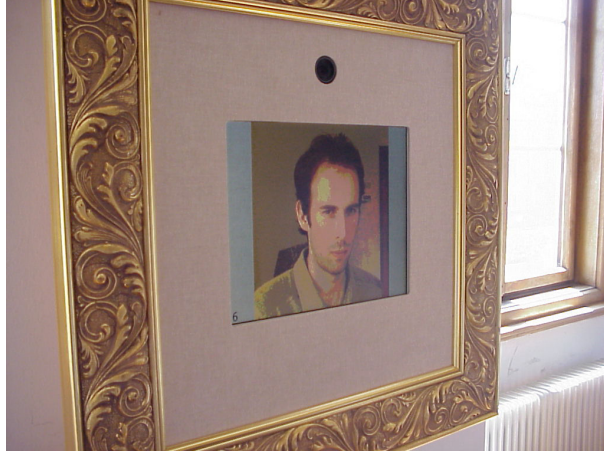
Figure 1: Computer monitor framed as a painting. Behind the round opening above the monitor is hidden a digital camera.
