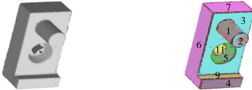
Figure 2: Generated intensity image of an object and its range image segmentation. Each description is labeled with a number.
